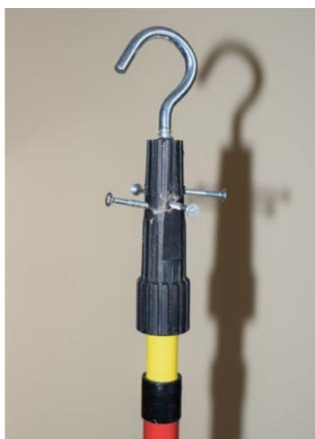
**Weed collector made from an extendable paint roller handle, large hook and four 2-inch no.8 screws. Materials purchased from the Range at total cost £3 (including packet of 2 hooks). The paint roller handle is 1m long, extending to 1.75m – another metre or so would be even better. It is made from iron, so is liable to rust after use. It is light enough to easily carry around but also strong enough to be used to bash emergent**
